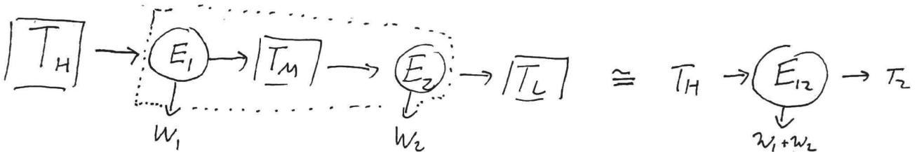
We can combine the two engines into one "super-engine" directly connecting the hottest and lowest points,  $T_H$  &  $T_L$ .
