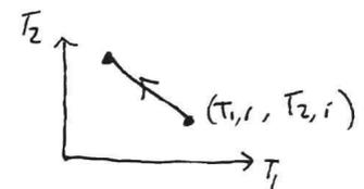
$$\Rightarrow \frac{dT_2}{dT_1} = - \frac{m_1 c_1}{m_2 c_2} \Rightarrow T_2(T_1) = T_{2,i} + \frac{m_1 c_1}{m_2 c_2} (T_{1,i} - T_1)$$
