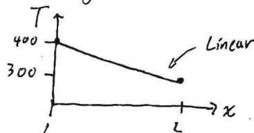
(b+c) When heat flows through the rod, in steady state, there is no net  $Q$  into the rod:
