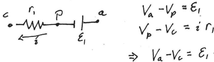
$$\begin{aligned} V_a - V_p &= E_1 \\ V_p - V_c &= i R_1 \\ \Rightarrow V_a - V_c &= E_1 + i R_1 \end{aligned}$$
