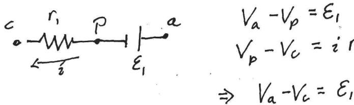
$$\begin{aligned} V_a - V_p &= E_1 \\ V_p - V_c &= i R_1 \\ \Rightarrow V_a - V_c &= E_1 + i R_1 \end{aligned}$$
