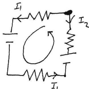
$$\begin{aligned}E_1 &= 2 \\E_2 &= 6 \\R_1 &= 2 \\R_2 &= 4\end{aligned}$$
