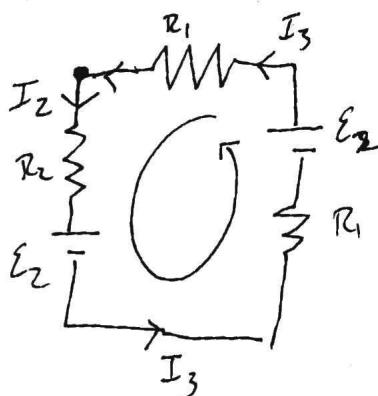
$$\begin{aligned}\textcircled{O} &= -I_2 R_2 - E_2 - I_3 R_1 + E_2 - I_3 R_1 \\&= -I_2 R_2 - 2 I_3 R_1\end{aligned}$$
