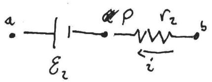
$$\begin{aligned} V_a - V_p &= E_2 \\ V_b - V_p &= i R_2 \\ \Rightarrow V_a - V_b &= E_2 - i R_2 \end{aligned}$$
