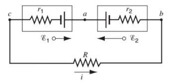
**2.** (*RHK Sample 31-3+4*) (a) Find the currents in the circuit below, if  $\mathcal{E}_1 = 2$ ,  $\mathcal{E}_2 = 6$ ,  $R_1 = 2$ ,  $R_2 = 4$ . (b) What is the potential difference between points a and b?
