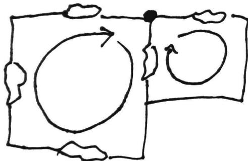
Loop: Directed path along some part of a circuit that ends where it starts
