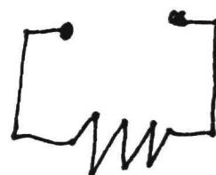
$$R_{\text{eff}} = r_1 + R + r_2$$
